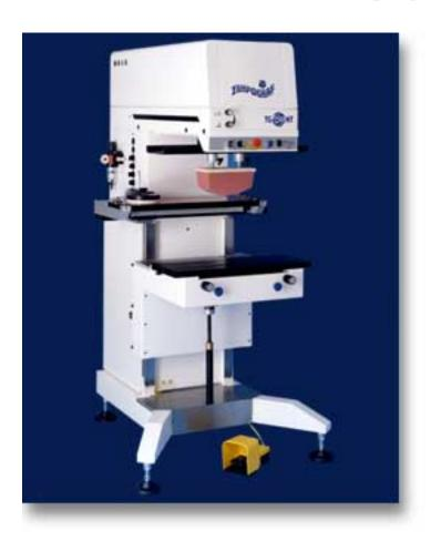
ADVANCED ELECTRO-PNEUMATIC OFFSET PRINTING MACHINES UTILISING FLEXIBLE IMAGE TRANSFER PADS.
